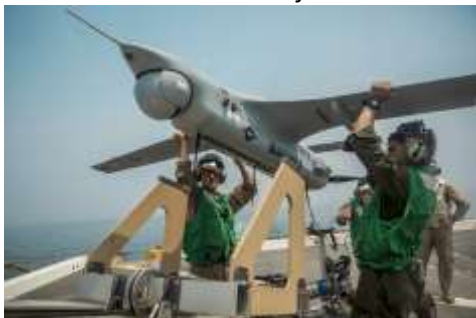
Marines lift an RQ-21A Blackjack unmanned aerial system onto a launcher before flight operations aboard the USS John P. Murtha in the Arabian Sea, July 31 2019.
