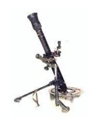
The M252 is a gravity-fired smoothbore system. Attached to the muzzle of the weapon is the Blast Attenuation Device (BAD), used to reduce the blast effects on the mortar crew. To increase cooling efficiency, the breech end is finned; though first-hand accounts attest that the level of cooling is negligible. The M252 system weighs 91 lbs. completely assembled and is composed of the M253 Cannon, M177 Mount, M3A1 Baseplate, and the M64A1 Sight Unit.
