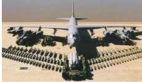
The B52H Stratofortress (also known as the BUFF, or Big Ugly Fat Fellow) has a weapons payload of more than 70,000 lbs.
