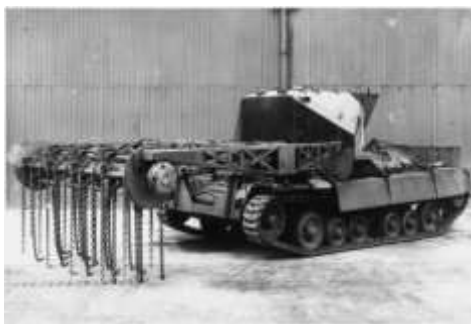
Experimental flail mounted on a Valentine tank; the Valentine Scorpion was never used operationally.
